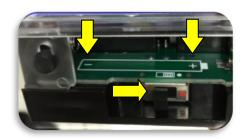
B. The battery ON/OFF switch is ON with the slider towards the right side (Red Dot) of the OxSim Flex.
